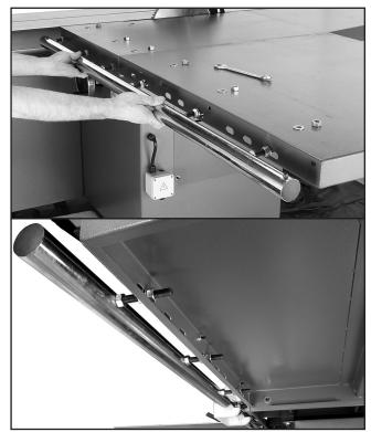
Figure 22. Installing the round rail.
